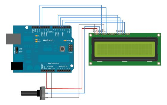
Fig. 3.3: Lcd display connections
