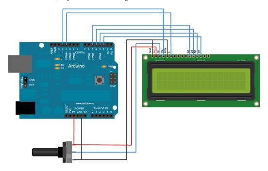
Fig. 3.1: Lcd display connections
